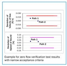
After assembly of the meter, a zero flow verification test is performed to verify proper transit-time measurement. Zero flow stability dominantly affects a meter's low-flow performance. The acceptance criteria for FLOWSIC600 zero flow verification exceeds the requirements from AGA9, and therefore ensures good low-flow performance.
