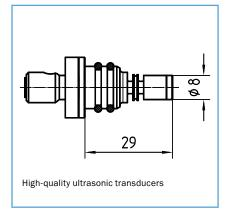
High-quality transducers are the heart of our intelligent measurement devices. All transducers are made of titanium, are hermetically sealed without a matching layer and wet gas protected. SICK transducers are subject to precise geometrical dimensional and impedance checks before they are matched pairwise to provide the utmost accuracy on each ultrasonic path for superior performance.
