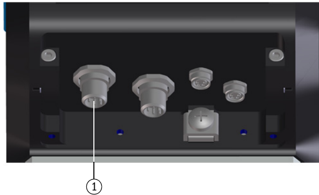
Fig. 19 Connection for external power supply underneath the meter cartridge
