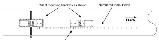
Refer to the Site Installation Details document provided with the installation hardware to determine the correct hole location.
