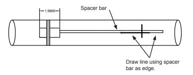
7. Wrap the Mylar spacing guide around the pipe so that the left edge is against the transducer edge mark. Arrange so that one end overlaps the other. Ensure that it is snug around the pipe and mark along the overlapping edge.
