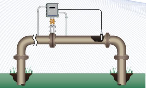
Reference Accuracy (Includes combined effects of linearity, hysteresis, and repeatability): ±0.075% of calibrated span or upper range value (URV), whichever is greater; Absolute Pressure Measurement: Upper Range Limit: 1,500 psia. Turndown Ratio: 15 to 1. Reference Accuracy (Includes combined effects of linearity, hysteresis, and repeatability): ±0.075% of calibrated span or upper range value (URV), whichever is greater - Terminal based.
