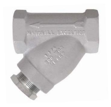
The ME650S Series Ductile Iron Strainers are available in standard pipe sizes with threaded blow-offs. All strainers come standard with 40 mesh stainless steel screens for maximum protection of equipment. Other mesh sizes are available upon request. Plugs for the threaded blow-offs are available at additional cost.\*
