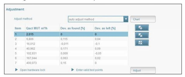
2. Enter by double clicking a sufficient number of test flow rates and the deviation to the reference meters in %. The software calculates the coefficients for the correction automatically.
