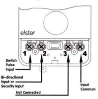
Note: Connections to reed-switch pulsers, such as AMCO Water Metering Systems' LRP (on the T3000) and T-probe for the V100 (red and blue wires), are made to pins 1 and 4. The security input requires a loop connection to the common input (between pin 2 and pin 4). A direction flag input is required for pin 2 and pulse input to pin 1 when used in a bi-directional mode.
