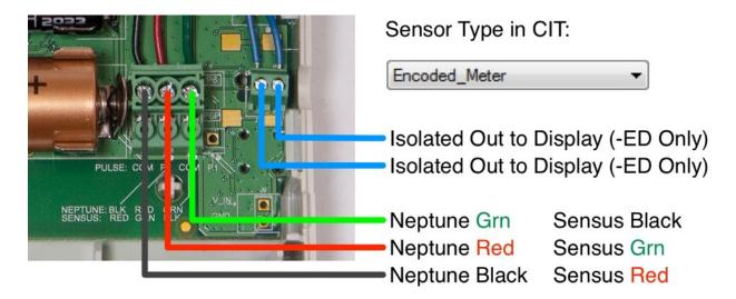
Our TW-140B-ED unit additionally provides a pulse output to drive a remote display as required in California. This output is a isolated dry-contact type and can drive any display that accepts this type of input. There is no polarity associated with this connection.
