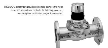
An electronic digital pulse output with the 4–20mA analog option is available for customers requiring both digital and analog outputs. Reverse flow indication is available with the high frequency forward/reverse pulse output option.
