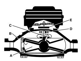
Liquid flowing through the meter chamber (A) causes a disc (B) to nutate or wobble. This motion, in turn, results in the rotation of a spindle (C) and drive magnet (D). Rotation is transmitted through the wall of the meter to a second magnet (E) which operates the transmitter.
