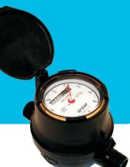
**Operation.** The C700 polymer meter is a positive displacement type meter operating on the oscillating piston principle. The product utilizes a piston that water use rotates in a measuring chamber, each piston revolution being equivalent to a known volume of water. The piston movement is transferred by magnetic drive to a straight reading sealed register which contains the appropriate reduction gearing.
