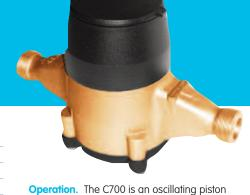
Operation. The C700 is an oscillating piston style, positive displacement water meter. The product utilizes a piston that water use rotates in a measuring chamber, each piston revolution being equivalent to a known volume of water. The piston movement is transferred by a magnetic drive to a straight reading sealed register which contains the appropriate reduction gearing.
