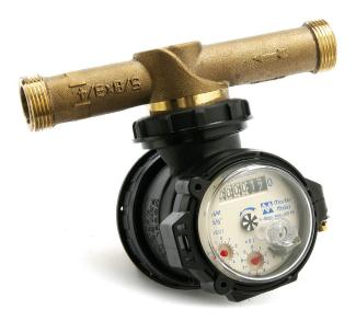
The next time you're faced with a challenging residential installation, check out the Master Meter flexible axis meter (FAM). FAM flow tubes can be installed horizontally, vertically, or any angle in between. No matter where it ends up, the FAM measuring chamber remains horizontal for accurate -- and quiet -- operation. It can also be positioned so it is always facing up for easy reading.
