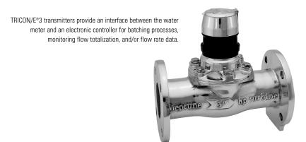
An electronic digital pulse output with the 4-20mA analog option is available for customers requiring both digital and analog outputs. Reverse flow indication is available with the high frequency forward/reverse pulse output option.
