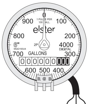
A maximum cable length of 50 feet is recommended, however cable lengths up to 500 feet are possible if shielded cabling is routed away from electromagnetic sources. Cable sizes from 24-32 AWG are acceptable. Wiring is not polarity sensitive (see schematic below).
