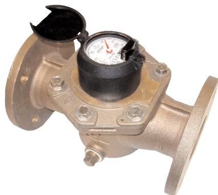
The Digital Register may be used with Elster AMCO Water's T4000 Turbine cold water meters, sizes 1 1/2" - 12" and TS4000, sizes 1 1/2" - 6". This register provides a volt-free reed switch closure for a specific volume of metered water (see specifications). The actual pulse resolution and units of registration are printed on the dial plate.
