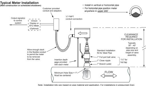
Note: Installation kits vary based on pipe material and application. For installations in pressurized (live) systems, use "Hot tap" 1¼ inch installation kit and drill hole using a 1 inch wet tap drill.
