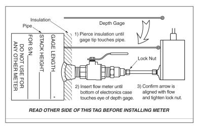
Prior to installing the meter, confirm that the stack height recorded on the tag is close to the actual stack height. Flow meter stems are intentionally over sized to allow for variations of at least 2" in the stack height. Contact ONICON prior to installation if there is any question regarding stack height or stem length. This way ONICON can offer you credit for your meter if you decide to exchange the meter for one with a different stem length. Returns may be subject to a restocking fee.
