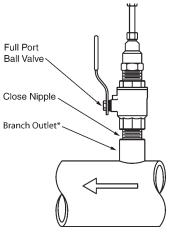
\*Weld-on fitting, copper tee or saddle
