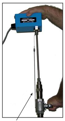
Step 2: Carefully withdraw the flow meter stem from the pipe until the sensor head is fully inside the hot tap adapter.
