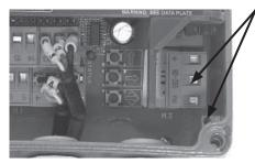
Step 6: Wire the connector as shown based on input type. Earth connection must be made.
