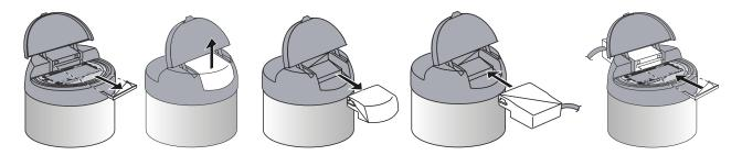
Do not hold the center of the retaining clip when inserting or removing it. Hold both ends and slowly insert or remove it. Ensure that that the lugs on the clip ends are pointed upward. Ensure the optical port is not blocked by foreign substances.
