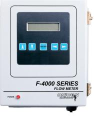
ONICON F-4000 Series Ultrasonic Flow Meters utilize the differential transit time method to measure the velocity of relatively clean liquids in full pipes. By measuring the difference between transit times of ultrasonic sound waves travelling between two transducers, the flow velocity and direction are accurately determined.
