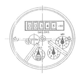
The 1800 Series counter consists of a row of numbers (roller counter) and one or more circular dials with rotating pointers. There is also a star shaped wheel that rotates whenever flow is present (trickle indicator).
