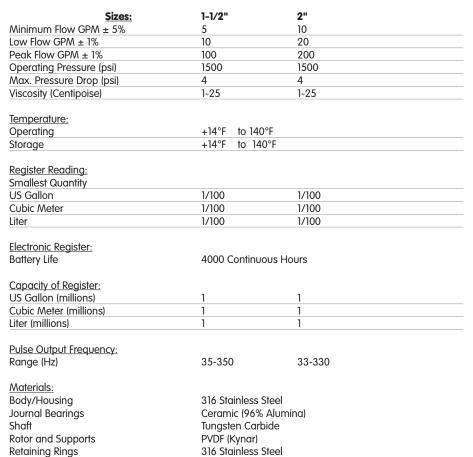
**Operation.** The 316 Stainless Steel Turbine meter is designed for those applications where a more rugged meter is required. The fluid passes through the meter without a change in direction, and drives the rotor in direct proportion to the quantity of fluid passing through the meter. Rotor revolutions are transferred to the electronic register by magnetic actuation of a pickoff coil.
