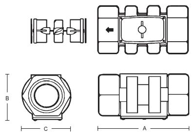
Note: Computer electronics add 0.7 in. (1.8cm) to height of turbine housing.
