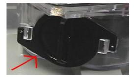
3. Remove both series (600143-001) batteries from the DATTUS meter without disconnecting them.
