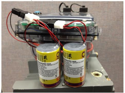
6. Place both batteries into the electronics enclosure, and seal them with the battery door.
