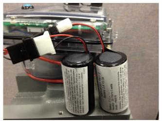
**4.** Replace each battery one at a time. Disconnect the first battery and immediately replace it with one of the parallel battery connectors. This ensures that the meter remains powered during the battery replacement.K
