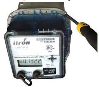
5. Carefully place the protective cover along the top meter edge.
