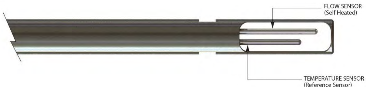
Figure 14 - One of the sensors is self-heated, and the other sensor measures the gas temperature.
