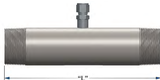
Figure 13 – The length of the flanged-flow body is the same as the NPT-flow body.
